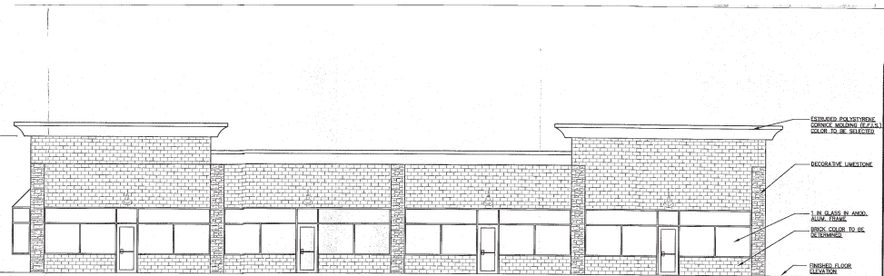
NORTH ELEVATION BUILDING 1 SCALE: 1/8" = 1'-0"
